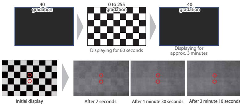
Fig.40 Result for residual image measurement
