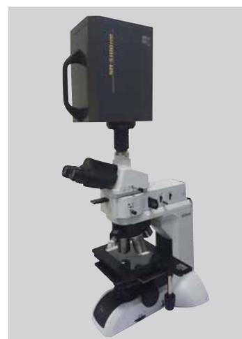
Fig. 7 SR-5100 + Metallurgical microscope
