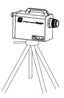
2 Remove the cap from the objective lens and set the finder shutter selection knob to "OPEN".
